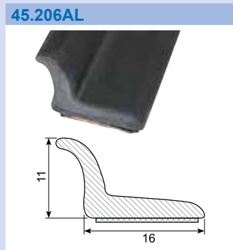
Material: PVC gutter with adhesive Length: 2 m
